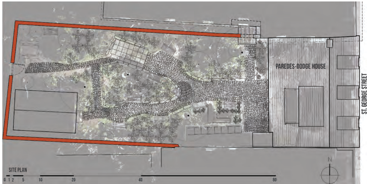
54 St George Street, St Augustine FL - Site Floodproofing example (walls shown in red)
