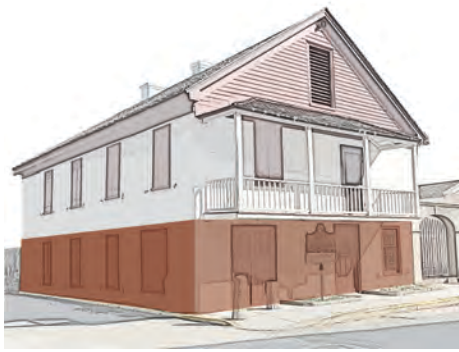
22 St Francis Street, St Augustine FL - Example of walls wrapped with a temporary waterproof membrane
