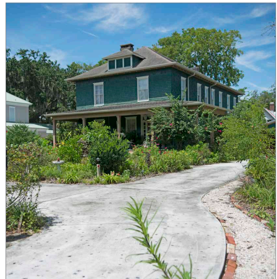
The gravel along the edge of this driveway and lush plantings reduces stormwater runoff by promoting absorption.
