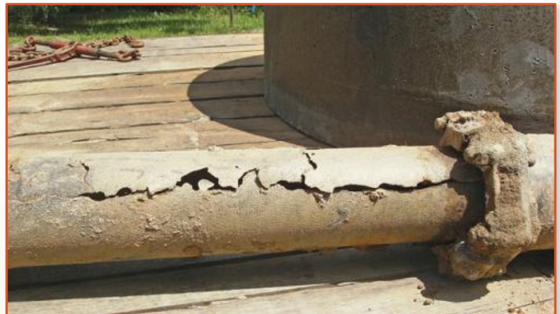
Deteriorated Ductile Iron Forcemain - Gwinnett County, GA
