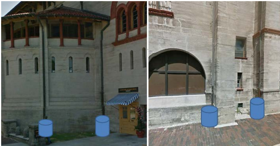
Figure 6-2 Potential locations for the installation of rain barrels at the City Hall building. Ideal locations are adjacent to pervious and vegetated areas for irrigation. Other areas should be considered as an educational tool to promote water reuse.
